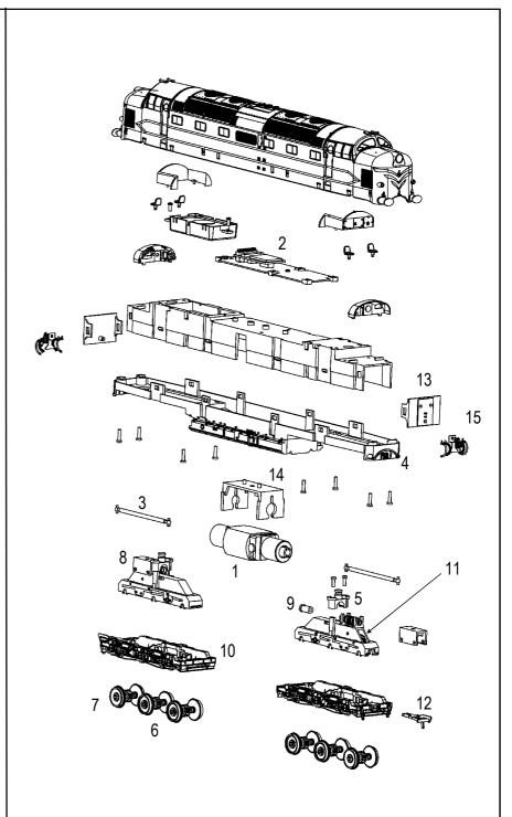
A DCC Sound fitted loco is shown. When fitting a sound decoder to a DC model, fit the speaker box in the cavity where shown.
